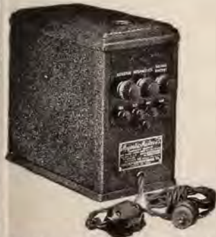
Above is seen the Majestic Master-B with a capacity of 60 milliamperes at 150 volts, suitable for use with Radiolas 25, 28 and 30
