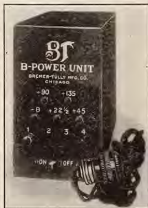
Bremer Tully's B power unit made for use particularly with their own receivers, but can also be used with other standard sets
