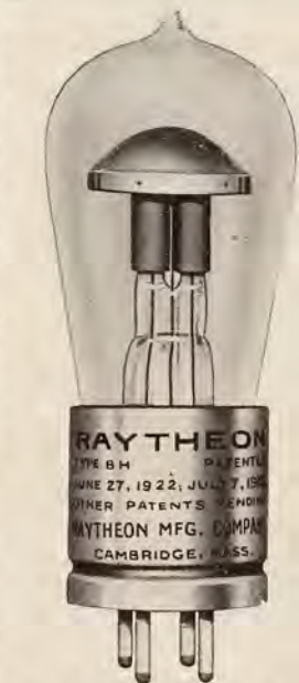
This is the new BH Raytheon tube which has a materially higher current and voltage output
