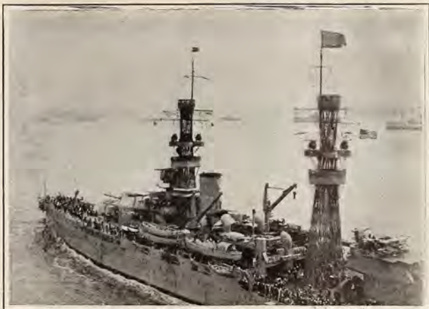
U. S. Navy battleship showing various radio antennas, each for a separate transmitter
