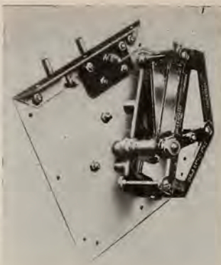
The Karas condenser is affixed to the under side of the meter panel
