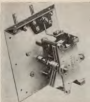
In this picture is shown the Cardwell condenser mounted on the under side of the wavemeter panel
