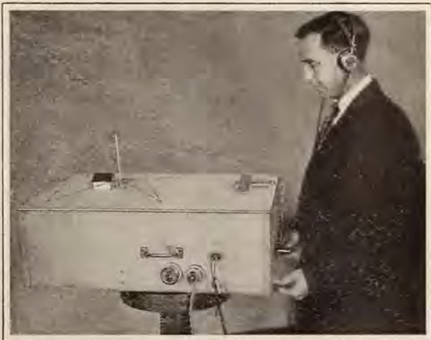
Model of double beam radio beacon developed in Radio Laboratory of the Bureau of Standards
