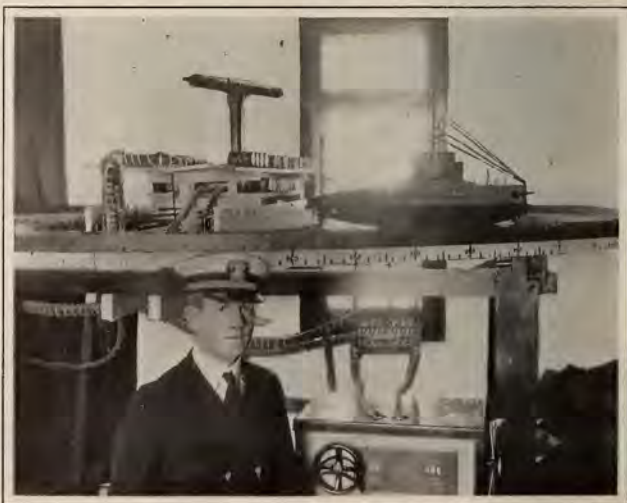
Naval radio direction finder with model submarine on test run
