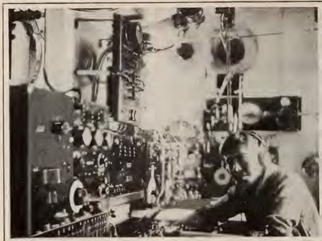
Typical scene in a U. S. Naval destroyer radio room. Receivers for all wave bands are shown as well as spark and tube transmitters
