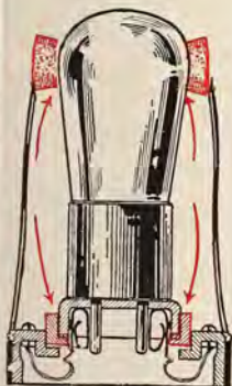
Showing double absorber for detector tube protection. The arrows point to the absorbing support between the base and the tube holder and to the damping side mufflers. Note the contact springs touch the tube prongs over a large area not making contact at one point only. This is UX Detector $1.00.
