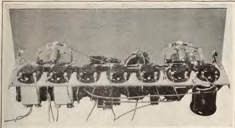
Figure 2 is the rear view of the seven tube portable showing the socket mountings all arranged in a line. The oscillator coil of the plug-in type is shown under the subpanel at the extreme right. All the long wave transformers are mounted underneath the subpanel as are the two audio transformers, the latter seen at the left of the picture
