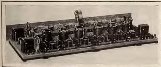
This is the Zenith set before the shielding is applied
