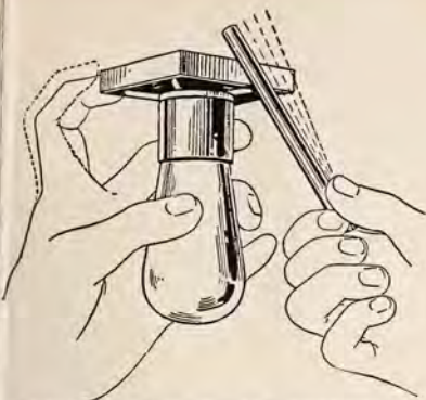
Tap the base of a spring-suspended socket and feel the vibrations. Then touch the base with finger and watch them disappear. This explains "snubber" action.
