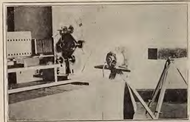
Radio Photo sending machine, lamp house to the left (for illuminating the picture); (2) four Prismatic Rings for moving the picture over the (3) light sensitive cell in the box at the right; time for each picture three minutes; distance limited only by power of the broadcasting station
