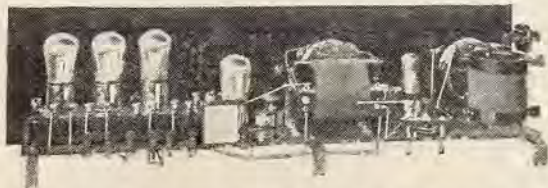
The picture above shows the use of an amplifier unit connected to the conventional receiver. Its use simplifies a good deal of the wiring and makes the set more compact.
