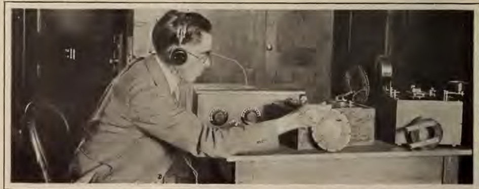
Morris S. Strock, of the Radio Laboratory of the Bureau of Standards, and the equipment designed for use by amateurs and broadcast listeners in measuring frequencies of a distant transmitter. By this method you can also calibrate your receiver
