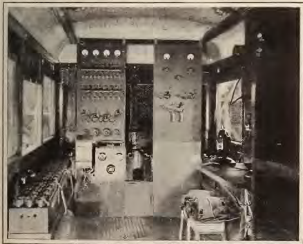
Warner Brothers' portable radio station 6XBR. Closeup of battery racks charging panel, generators and power panel.
