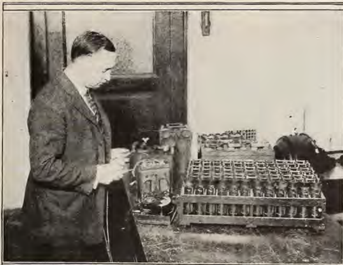
The author is shown making voltage tests on two kinds of wet batteries, the sulphuric acid and the alkaline type.
