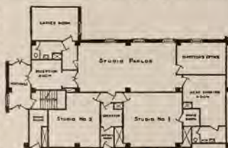
The above diagram illustrates the manner in which the studios, parlors and offices are arranged in the new studio of WJJD, located on the twenty-fourth floor of the Palmer House.
