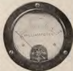
In testing work, and also for your own information, a milliammeter is quite desirable to determine the total plate current being used. If you are swapping hook-ups and changing tubes all the time, all the more reason for having a milliammeter in series with the negative B lead so as to read total space current.
