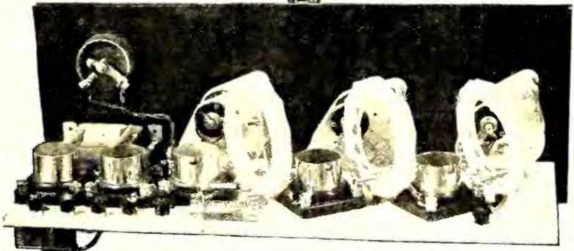
In the set above is shown the proper arrangement of coils to prevent inductive coupling. Engineers have made a study of the effect of the magnetic fields of adjacent coils upon each other, and efforts have been made to so place the coils in the receiver that the effect is reduced to a minimum. Radio experience also has shown that better results are obtained in reception if the aerial is pointing toward or away from the sending station sought. This is especially true of the loop aerial.
