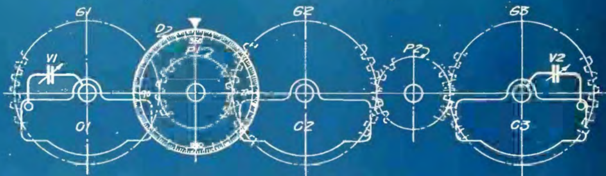
FIG. 3 REDUCTION GEARED CONDENSERS WITH A SINGLE 360 DEGREE DIAL CONTROL.
