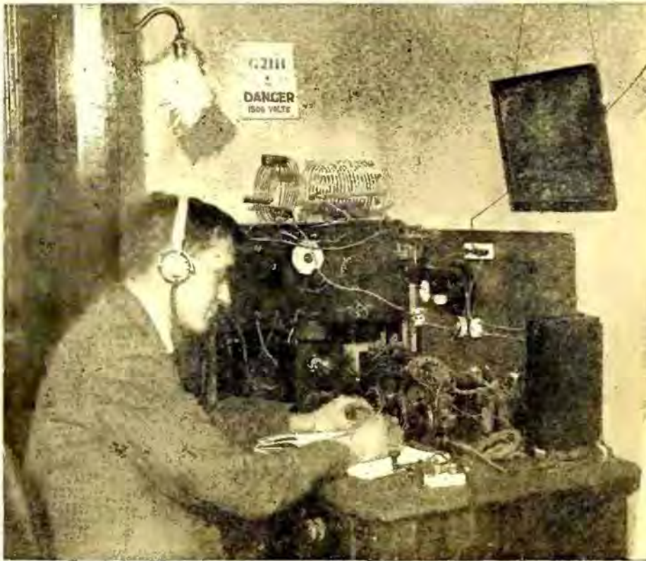
Fig. 1. The picture above shows Herbert Hiley, of the British station G21 H, situated at Keighley, Yorkshire, who has been successful in establishing communication with M. Fresni, Rua Aswaldo Cruz, Nieteroky, Brazil, a distance of 5400 miles with a wavelength of 42 meters and 15 watts in the antenna, the circuit used being a Hartley loose coupled. Mr. Hiley is shown logging a station. The photograph is by courtesy of G. Crowther, 28 Cark Road, Keighley, England.
