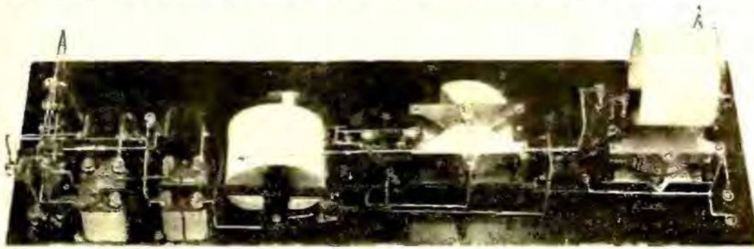
Fig. 1 Rear panel view of set described by Mr. Silver. All apparatus is mounted on the panel, there being no need for a baseboard.
