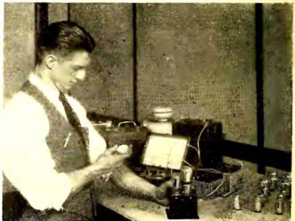
How a tube rejuvenator works. Such an instrument will renew the 201A and 301A as well as the UV199 and C-299 tubes in less than eleven minutes, it is claimed. As no meters are necessary, hosts of fans will find this set easy to build.
