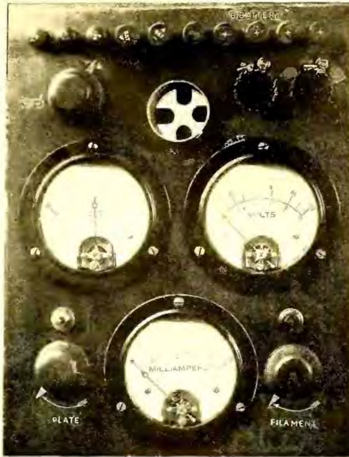
Fig 1. A front view of the vacuum tube tester, which can be made by any fan. Each part is so placed to give maximum efficiency, and no parts are used that will not be necessary. The tester is compact as well as attractive, and may be constructed for portable or stationary use.
