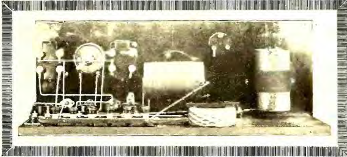
A front view of Mr. McCullah's much-discussed radiation-minimizing receiver. After a series of tests, Mr. McCullah believes he has nearly approached the ideal regenerative set with this four-tube hookup.
