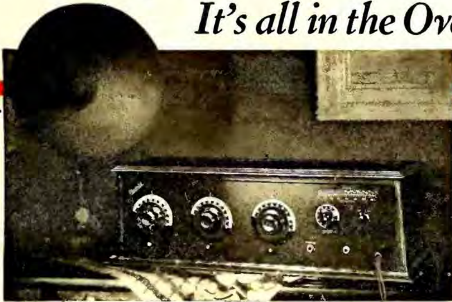
A 5-tube Receiver using the new Pfanstiehl system of tuned radio frequency
