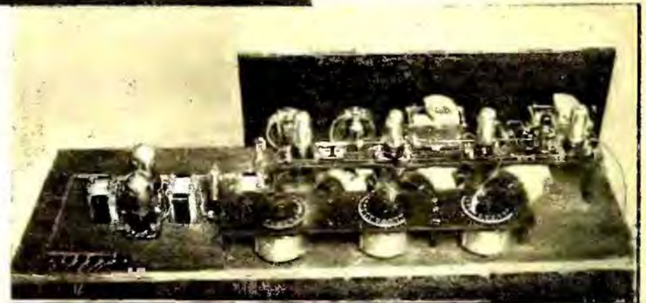
A rear view of the Sure-Shot super. Note how the cable connections, condenser mountings, etc., are made.
