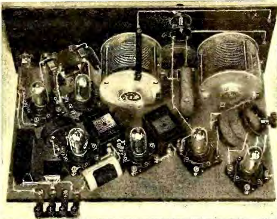
The business end of the powerful little superheterodyne receiver described by Mr. Green. It gives one an idea of what a compact efficient super-het should look like.
