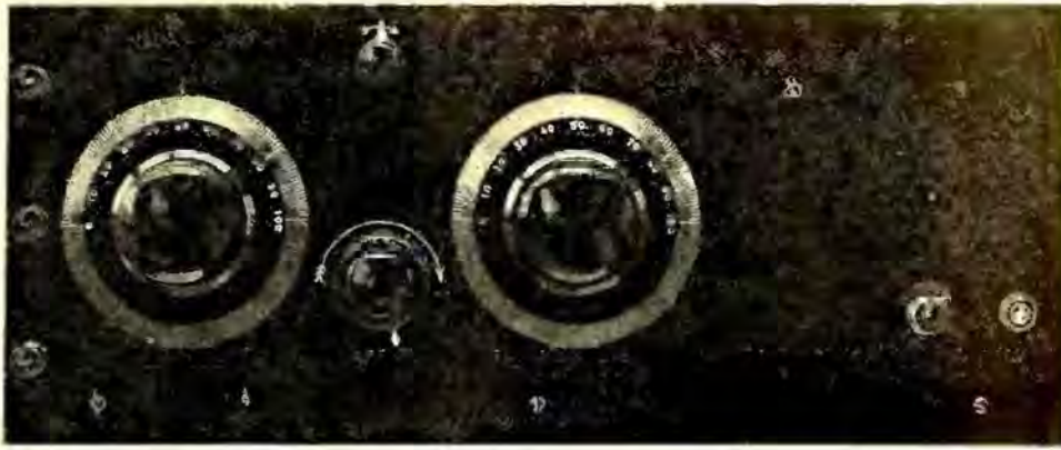
Two controls that require only two hands to tune with. The filament rheostat may be set and left there, and while the regeneration requires an occasional touch when tuning on widely separated wavelengths, it is not troublesome. The filament switch on the right permits one to turn off the set while lashing the phones or loud speaker to the table when strong signals are to be received.
