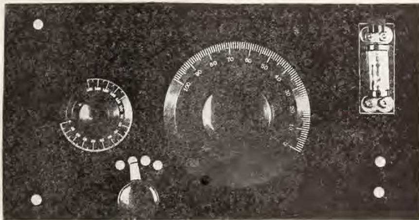
A front panel view of the beginner's crystal receiver, showing the simplicity of the panel layout.
