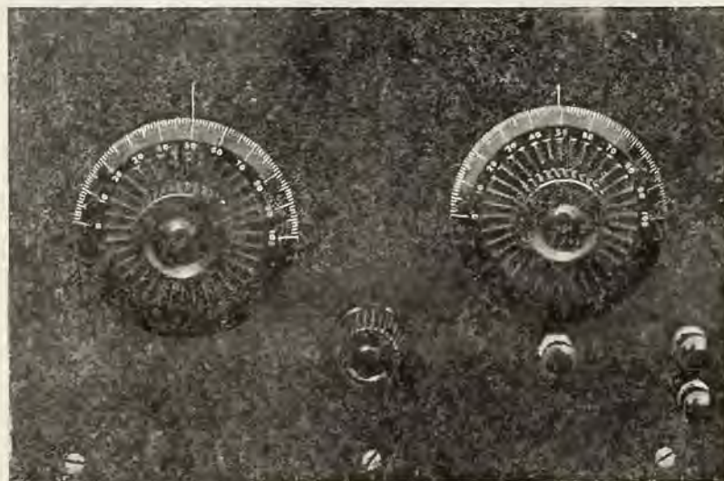
Fig. 3—A simple three-circuit set, front view. The rheostat knob is in the center, regeneration and tuning controls at left and right respectively, and phone binding posts at the extreme right.
