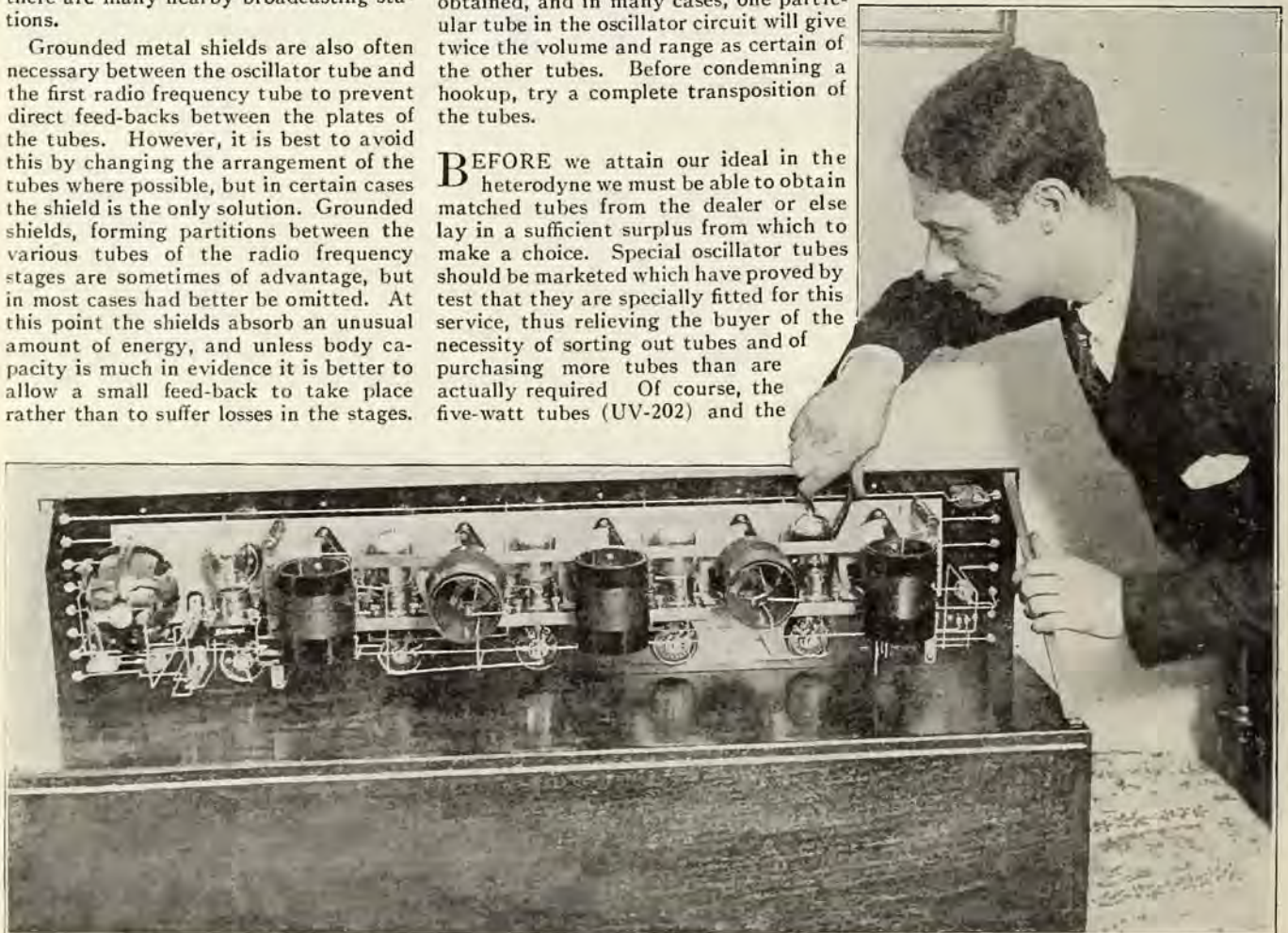
A rear view of a novel neutrodyne receiver constructed by a well known Eastern amateur radio builder, which shows some unusual feats of engineering skill. Note the method of off-setting magnetic coupling between the neutroformers, and the simplified arrangement of the receiver as a whole. The panel is shielded carefully from stray capacity effects, which may be introduced while operating.
