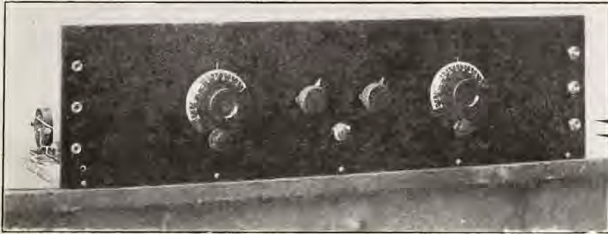
Photograph of the assembled super-heterodyne. Note the absence of numerous controls as commonly found on other eight tube Super-Heterodynes. Mr. Green has made the set simplicity itself and uses but two controls in the operation of the whole set.
