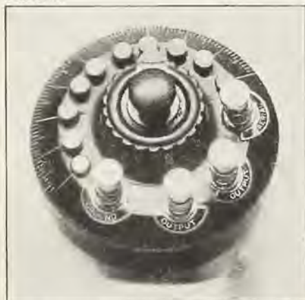
A top view of the "Dial Crystal Receiver" showing the arrangement of the taps, binding posts and illustrating the manner in which the vernier knob of the condenser dial is used as the switch knob to vary the inductance.
