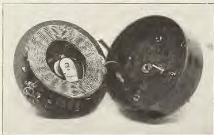
A view of the receiver "exploded" to show the manner in which the inductance is mounted. The crystal detector is mounted on case to the right, the mounting posts being visible in the photo.
