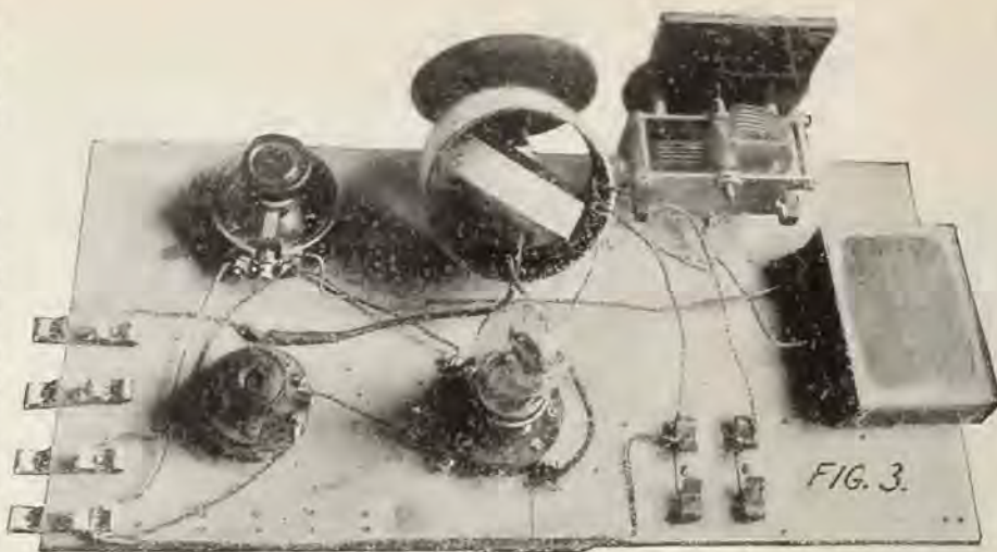
Figure 3. A board layout of the three coil tickler set which uses no grid condenser. The potentiometer and the C battery adjust the grid to the proper working potential.
