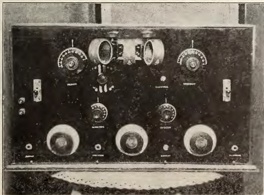
A closeup of the combination three-circuit honeycomb and neutrodyne set. (Kadel & Herbert.)
