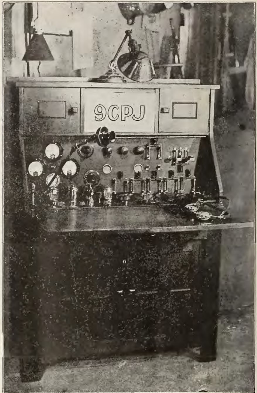
Station 9CPJ, built and operated by Charles G. Pelton of the Black Hawk Electric Company, of Waterloo, Iowa. 25 Watt C. W. 10 watt phone. With the receiver Mr. Pelton has picked up California, Canadian and New York stations.
