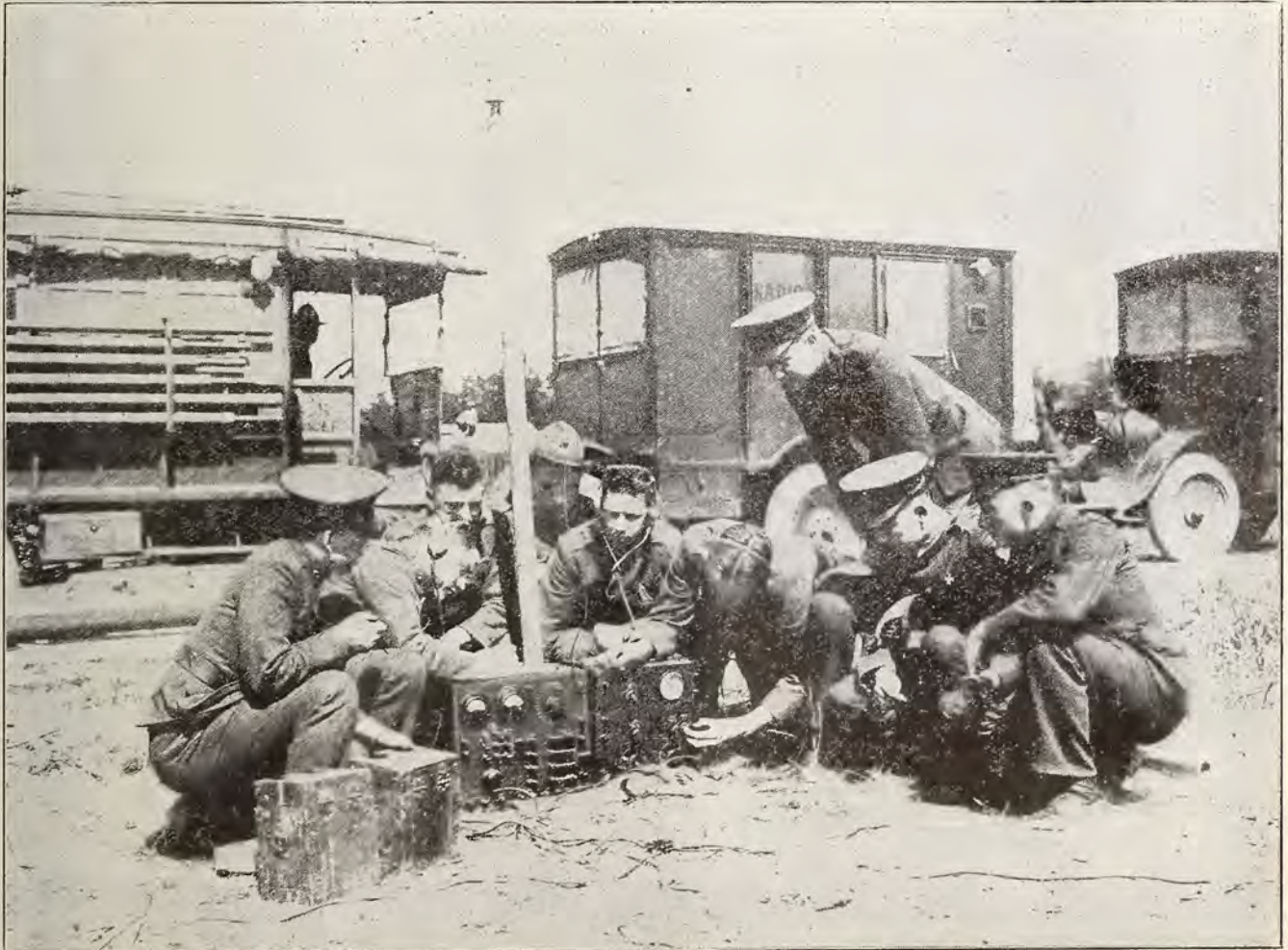
U. S. marine radio experts held their annual maneuvers near Waynesboro, Va., in September. They can place this field set, with its forty-five foot aerial, in position and have it in full operation in less than two minutes. They have equipped trucks, airplanes and tanks with radio. Official Marine corps photo.
