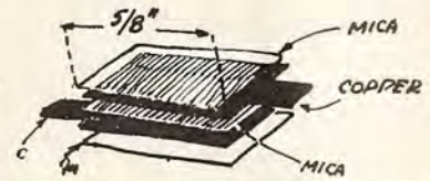
Figure 1. By this arrangement, the correct capacity for the .00005 MF condenser used in the Kaufmann circuit can be obtained.
