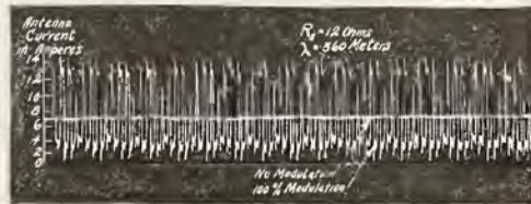
Fig. 5—Oscillogram of Rectified Antenna Current for Modulation of Vowel A
