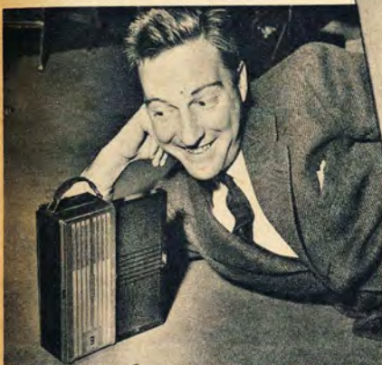
RCA VICTOR PERSONAL (BP-10). "Club Matinee's" Garry Moore uses this camera-type set of black fabrikoid and chromium, small enough to fit in overcoat pocket. Radio includes four tubes, three-inch speaker, "B" battery and flashlight cell. $20.00
