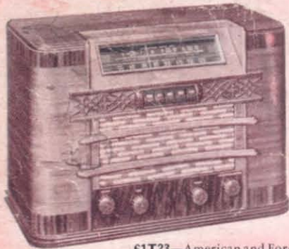
61T23—American and Foreign Reception—6 Tubes inc. rectifiers—3 Gang Condensers—5 Electric Push Buttons.
