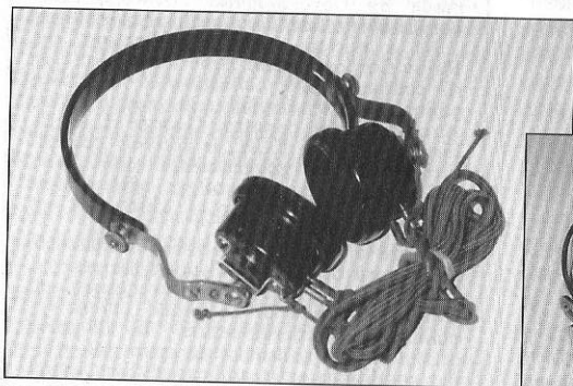
Wireless Specialty Apparatus adjustable diaphragm phones, circa 1910.
