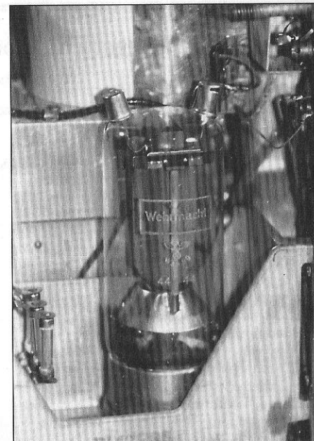
Closeup of one of the RL12P35s shows Wehrmacht identification.
