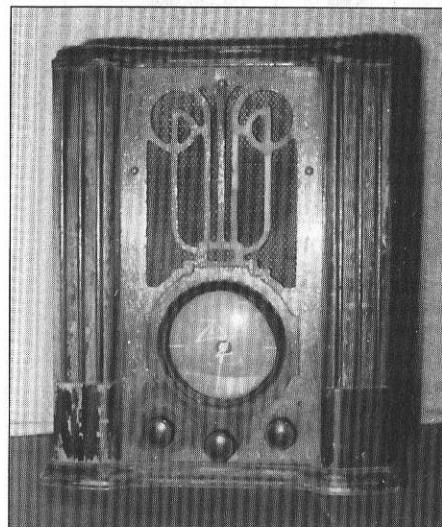
The 4V31 as found. Most of the grill veneer was missing.
