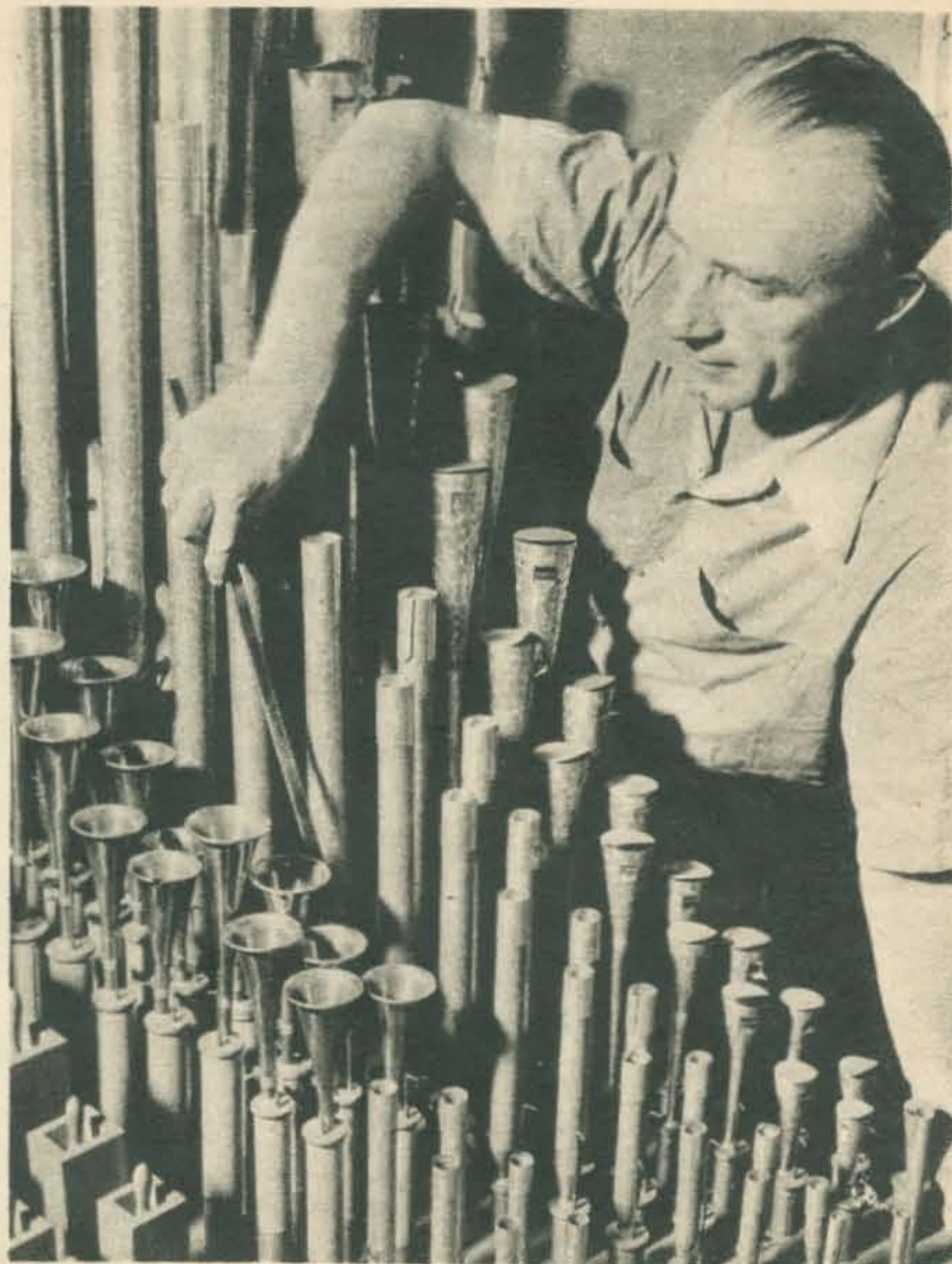
Pipe organs need the "doctor" only once a week. Art Nelson is shown using a steel rod to adjust small vents of the woodwinds.
